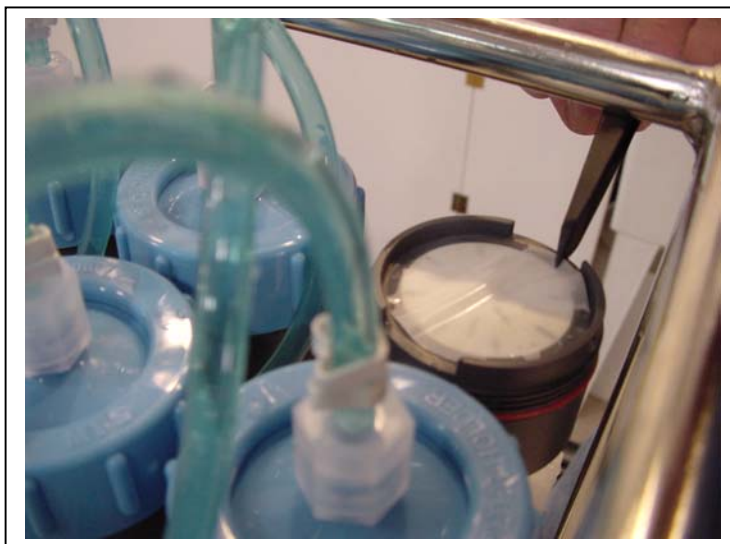
Figure 5-6: Placing Filter on Top of Frit
